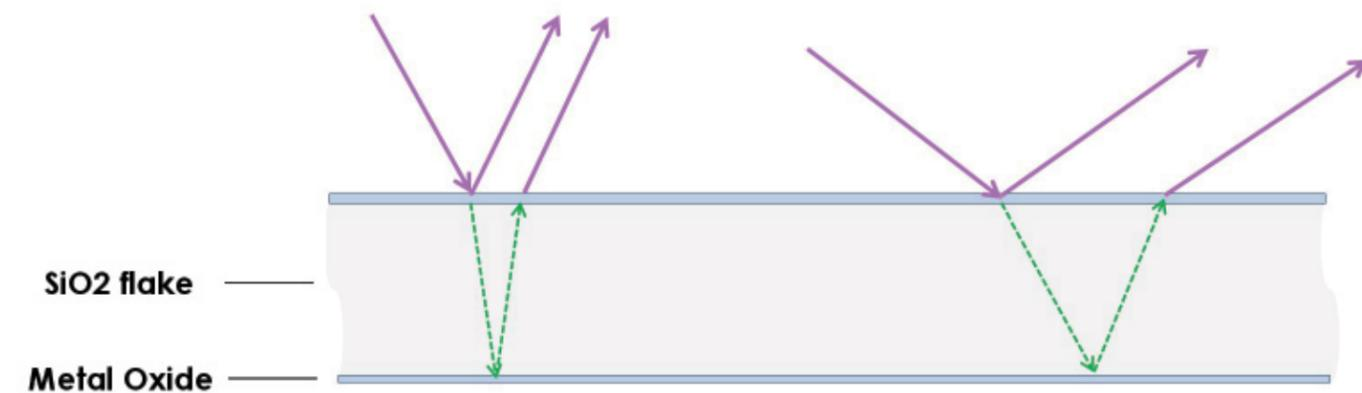
Due to the **thickness of the silica layer**, the **path length (directly related to the color)** of the reflected light differs significantly. If the incident light is at a sharper or wider angle, **the reflected light will have differing wavelengths of reflected light => different reflected colors.**
