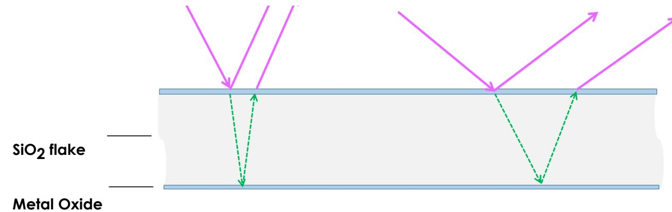
Due to the **thickness of the silica layer**, the **path length (directly related to the color)** of the reflected light differs significantly. If the incident light is at a sharper or wider angle, the **reflected light will have differing wavelengths of reflected light => different reflected colors**.
