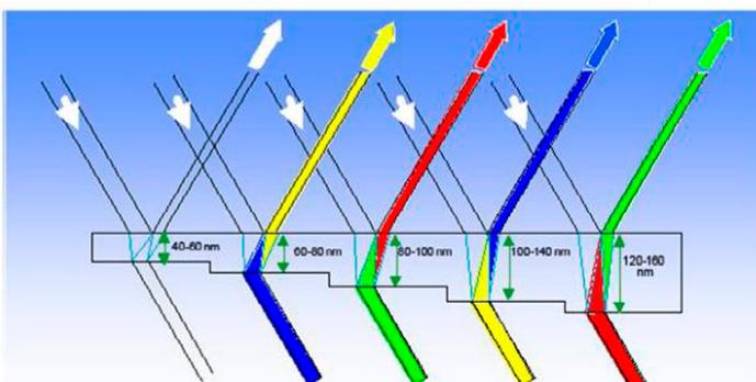
Thickness of the metal oxide layer determines the (reflected) interference color.
